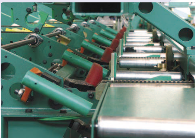
View of selection, alignment and orientation system for tubes and sections
