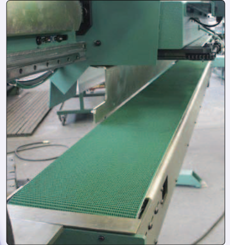
Motorised belt for multiple area unloading
